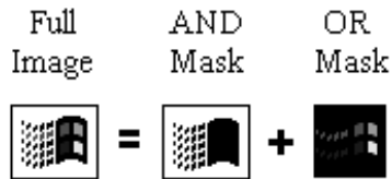
Figure 9-2: The icon and cursor image is a composite of an AND mask and an OR mask
